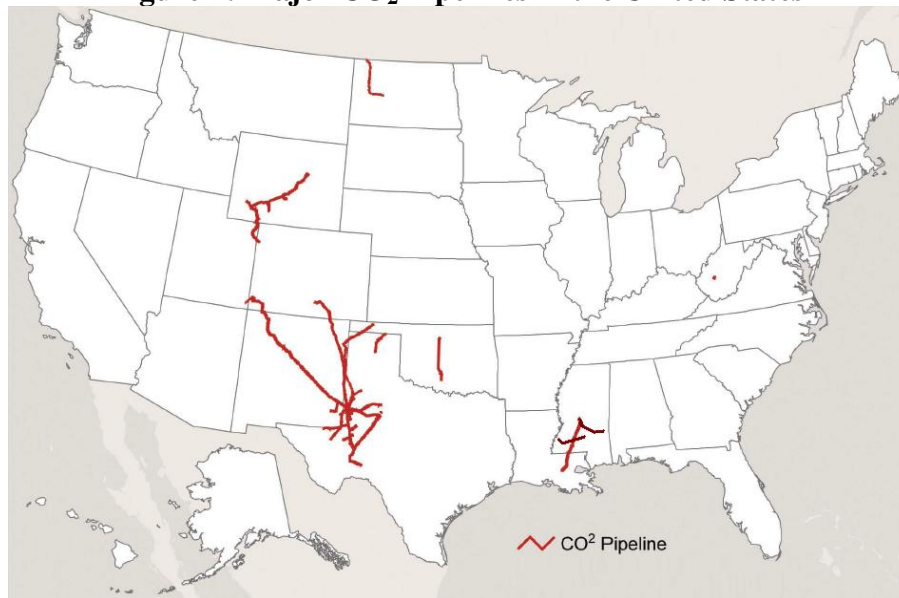
Figure 7: Major CO 2 Pipelines in the United States
